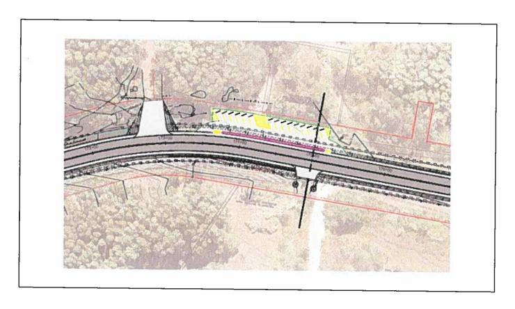
Five-foot paved shoulders and clearing up to the edge of the 100-foot right-of-way
